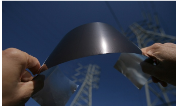
Fig. 4 - Example of Nanosolar's flexible solar cells.
