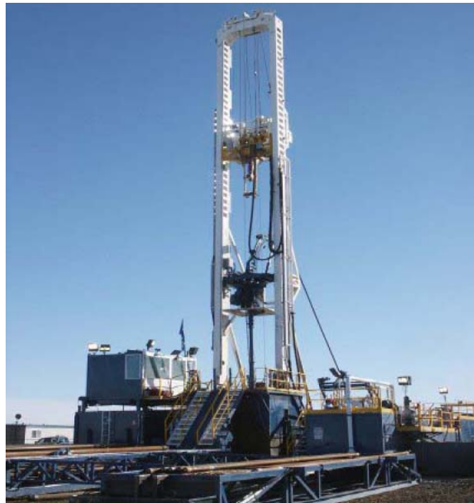
Fig. 1 – HCTR units have a relatively small size compared to a conventional drill pipe rigs, thus reduce environmental impact.
